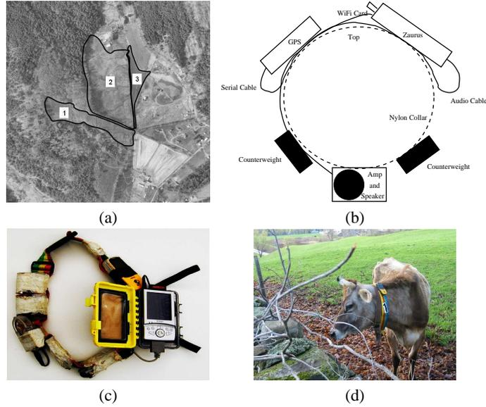
**Fig. 1.** (a) Aerial view of Cobb Hill farm. The fields where experiments were conducted are outlined in black. North is up. The photo displays an area approximately 1 km on a side. (b) The components of the Smart Collar include a Zaurus PDA, WiFi compact flash card, eTrex GPS, protective case for the Zaurus, an audio amplifier with speaker, and various connecting cables. (c) A fully assembled Smart Collar, with PDA case open. (d) A cow with a collar.
