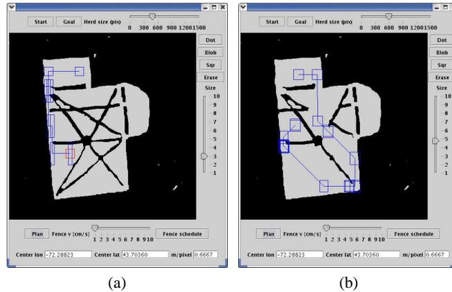
**Fig. 3.** GUI for dynamic fence planning. Environment is based on the Dartmouth Green, with some real-world paths defined to be obstacles. In (a), finding a path from the start (in top portion of free space) to the goal (at lower left) requires a significant change in the size and shape of the virtual paddock. (b) A more complex path — note that small overlap with obstacles is considered acceptable as long as sufficient free space remains in the virtual paddock.
