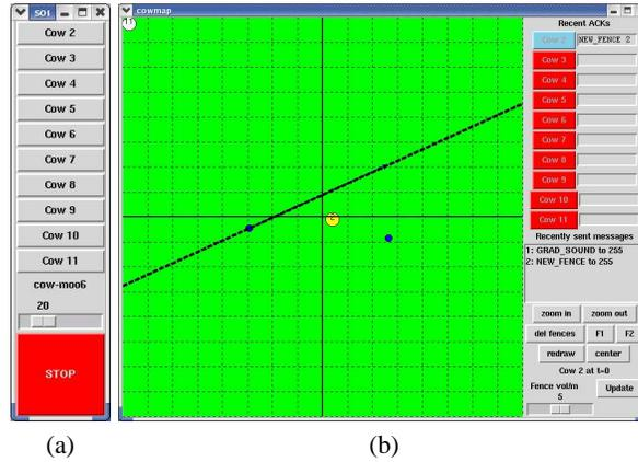
**Fig. 2.** GUIs used on laptops to monitor field experiments. (a) Sound control GUI. Pressing a button triggers the current sound on a specific cow. Current sound and volume can also be selected. (b) Map control GUI. Shows the last reported position of each cow, whether it is currently playing a sound, and whether an Alive message has been received recently. Buttons and text boxes in upper right show recent command acknowledgments from collars.
