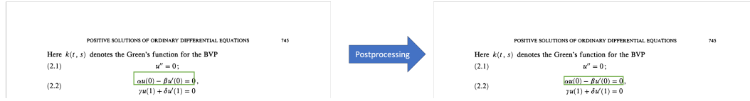
Figure 3.6: Example of postprocessing of a box so that it perfectly fits the connected components inside it or connected components it is touching
