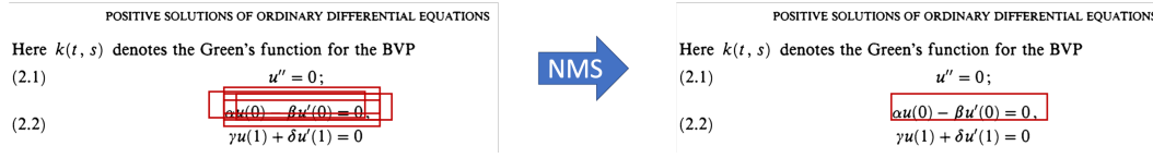
Figure 2.1: Example of NMS. The left image shows multiple detections for one math expression and right image shows the output generated after NMS.
