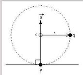
The inverse of the radius ( $r$ , in mm) of the largest circle in the set of circles containing a point ( $p$ ) and each neighbour ( $q$ ) of  $p$ . Circle centers are located along the point normal ( $n$ ) of  $p$ . Circles lie in the plane defined by  $p$ ,  $q$ , and  $c$  [3].
