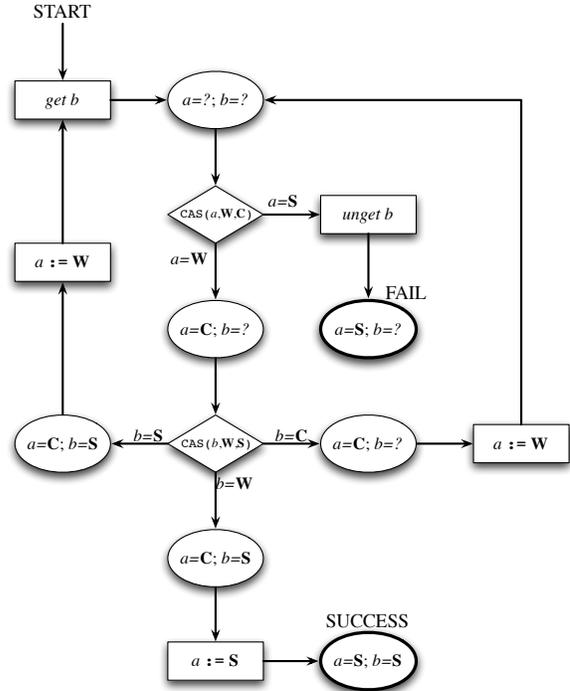
Figure 9. State diagram for the `blockFn` protocol
