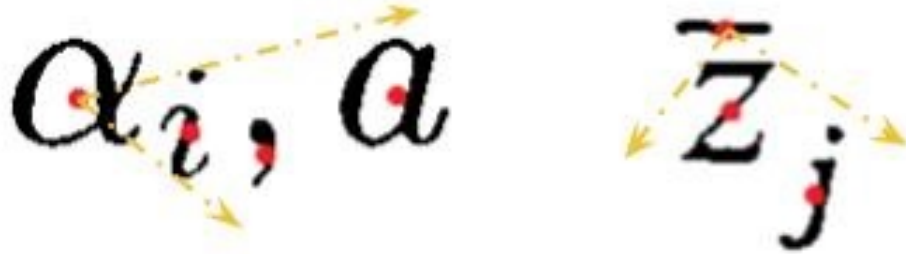
Figure 3.7: Examples of blocked line of sight. (Left) The subscript i symbol is blocking the line of sight from the alpha to both the comma and a symbols. Because the i symbol is closer the angle range it blocks is removed from the visible range before the alpha looks to the comma or a. (Right) The z symbol blocks line of sight between the overline and the j symbol. In the original graph structure that ' j ' would be a subscript to the overline accent. After restructuring the j is a subscript to the z instead.
