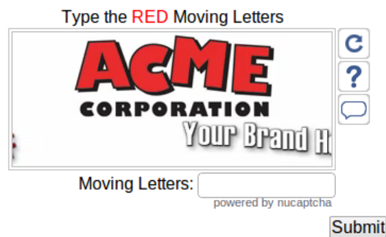
Figure 2.2: An online demonstration of the NuCaptcha video CAPTCHA service. The text shown in red is animated, and must be entered correctly for the test to be passed.
