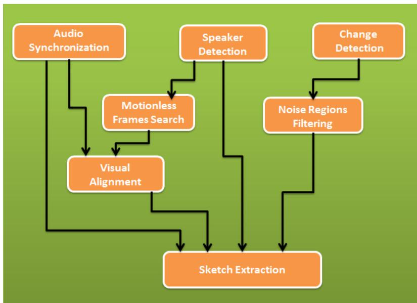
**Figure 10.** Tasks involved in the first process of converting the input videos into region of content or sketches that will be indexed by later process. Note that certain processes like audio synchronization, speaker detection, and change detection could be executed in parallel as they do not depend on any other task, but the later tasks have dependencies on the results from the previous tasks.
