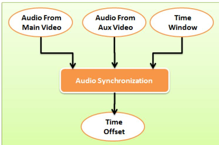
**Figure 11.** Process of synchronization of videos which is done by aligning their audio streams. An additional parameter that limits the range of the search for the best alignment is required and the result is a time offset that must be applied to the auxiliary video to match the timing in the main video.
