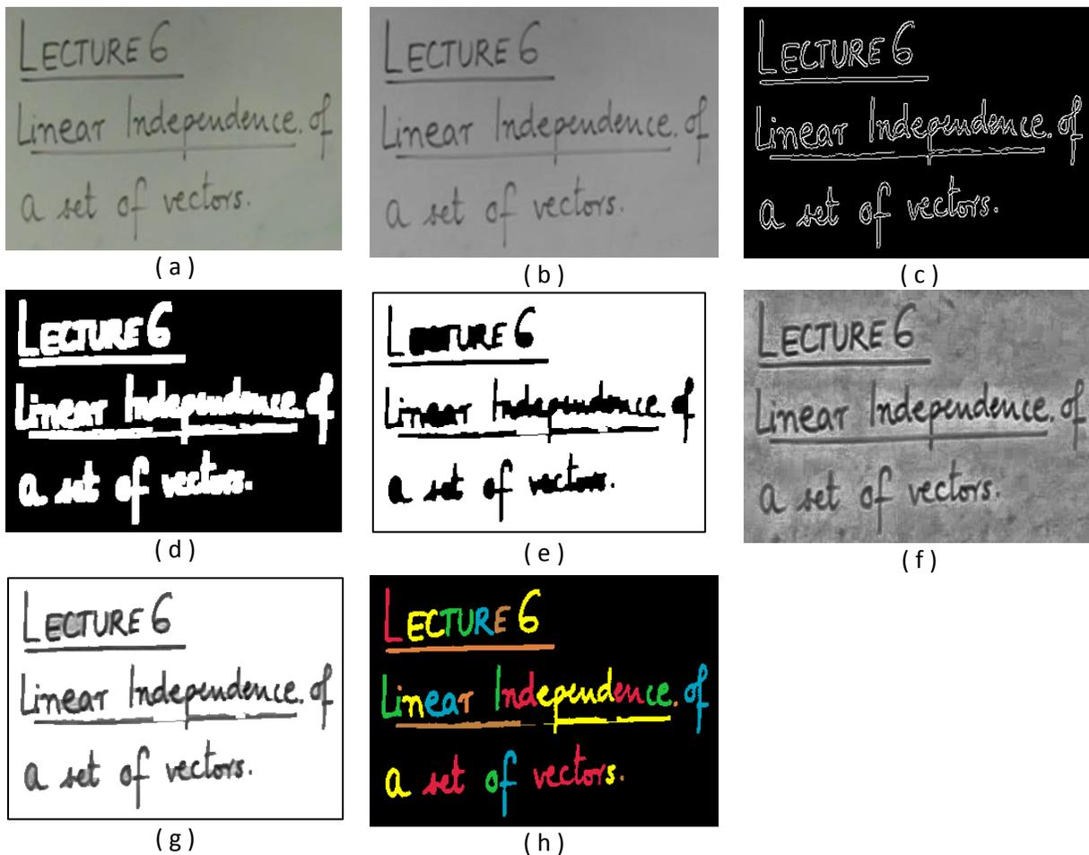
**Figure 28.** Steps to extract connected components. ( a ) input image, ( b ) converted to grayscale, ( c ) Edge Detection, ( d ) Dilation of edges, ( e ) Whiteboard Mask, ( f ) Adaptive Histogram Equalization, ( g ) Applying the mask ( e ) to equalized ( f ), ( h ) final connected components after labeling.
