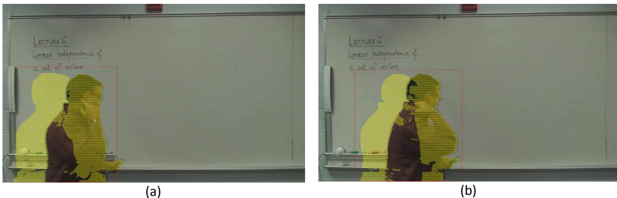
**Figure 19.** Some examples of the speaker detector algorithm. The Yellow pixels represent subsampled pixels where motion was detected. The red box represents the area where the speaker is believed to be present based on the center and standard deviation of the pixels with motion. (a) and (b) are two contiguous subsampled frames.
