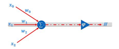
This calculates activation value of single (output) unit that is connected to 3 (input) sensors.
