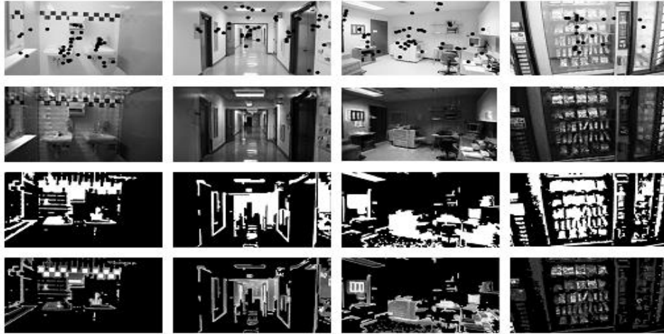
Figure 4: Sample input images with overlaid fixation plots ( 1^{st} row) – from left, washroom, hallway, office, vending. Low-level saliency maps ( 2^{nd} row), proto-object maps ( 3^{rd} row), and final conspicuity maps ( 4^{th} row).
