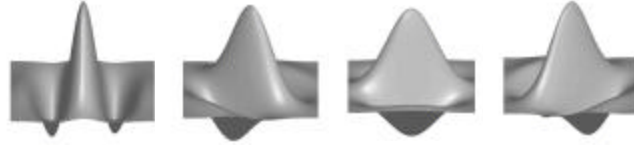
Figure 2 Basis functions of the Gabor filters used to detect oriented edges. From left, 0°, 45°, 90°, and 135°.
