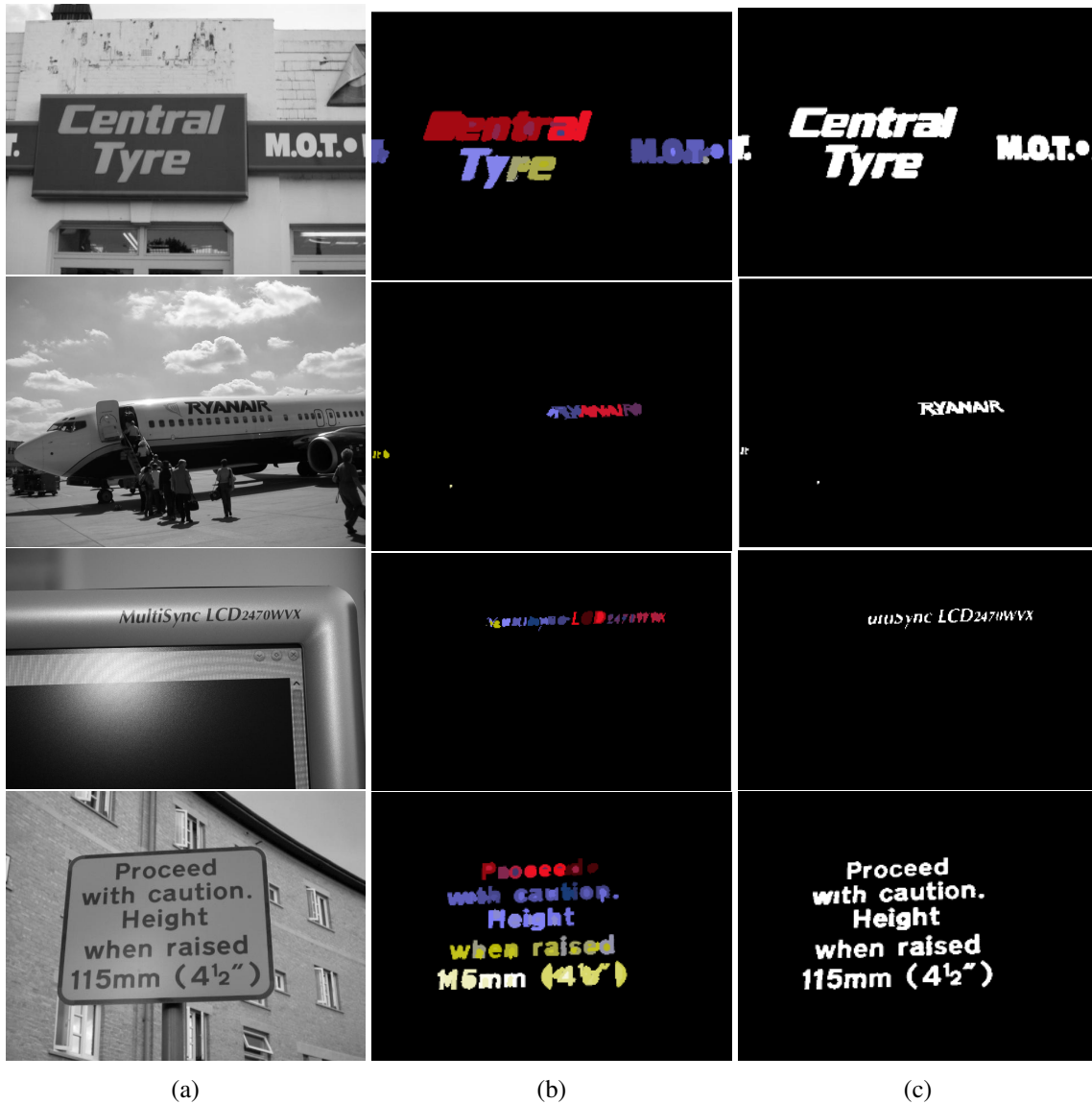
Figure 6.4: Examples of region growing and validation to form CCs. (a) The original image; (b) The detected CCs after patch based coarse and fine detection, and region growing with multiple parameters are used to generate candidate CCs; (c) The validation AdaBoost classifier is used to trim background CCs from the image and the final pixel level detection map is formed.
