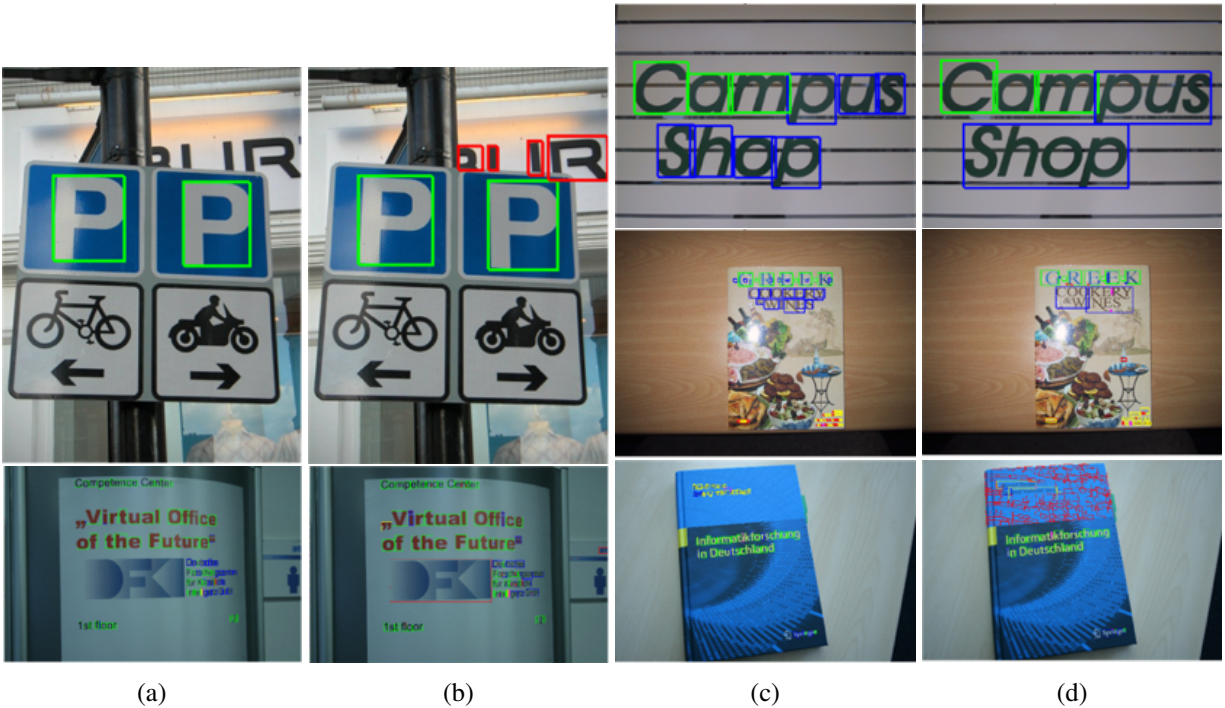
Figure 6.10: Example of character bounding box evaluation results. The character bounding boxes are evaluated with ground truth provided by ICDAR. The left column indicates the ground truth bounding boxes while the right indicates the predicted bounding boxes. The evaluation follows the method that was provided by [1]. Green boxes indicate perfect matches. The blue boxes indicate one-to-many under-segmentation of prediction, where characters are connected into larger bounding boxes. Magenta bounding boxes indicate the prediction has low recall, but acceptable precision. Where yellow indicates low precision but good recall. The red bounding boxes indicate a wrong detection.
