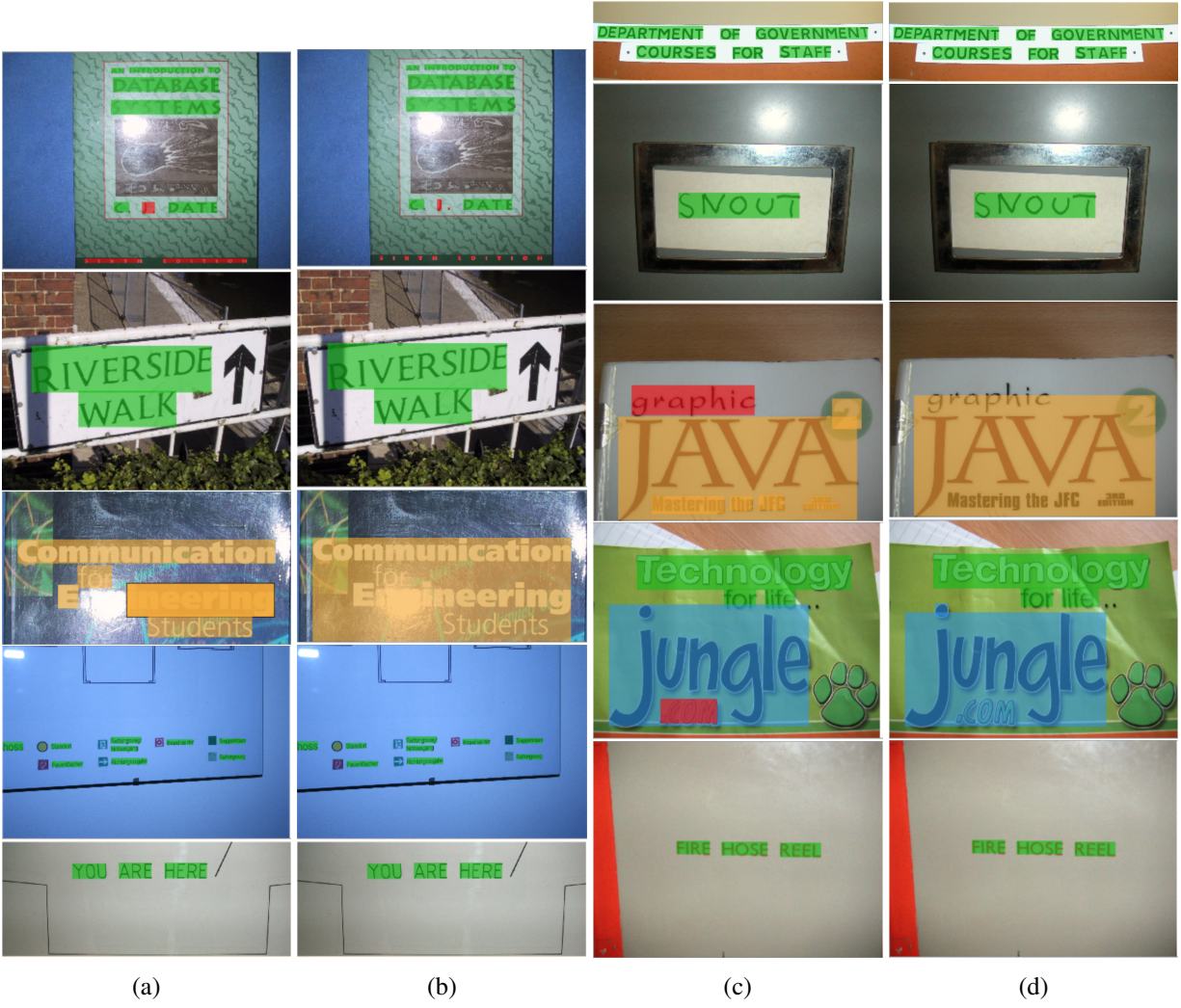
Figure 6.16: Examples of character bounding box evaluation results with comparison of ground truth and detections. (a)(c) are ground truth bounding boxes; (b)(d) are prediction bounding boxes. Red bounding boxes represent missing and false positives, green bounding boxes represent correct detections, yellow bounding boxes represent under-segmentation, and blue bounding boxes represent over-segmentations.
