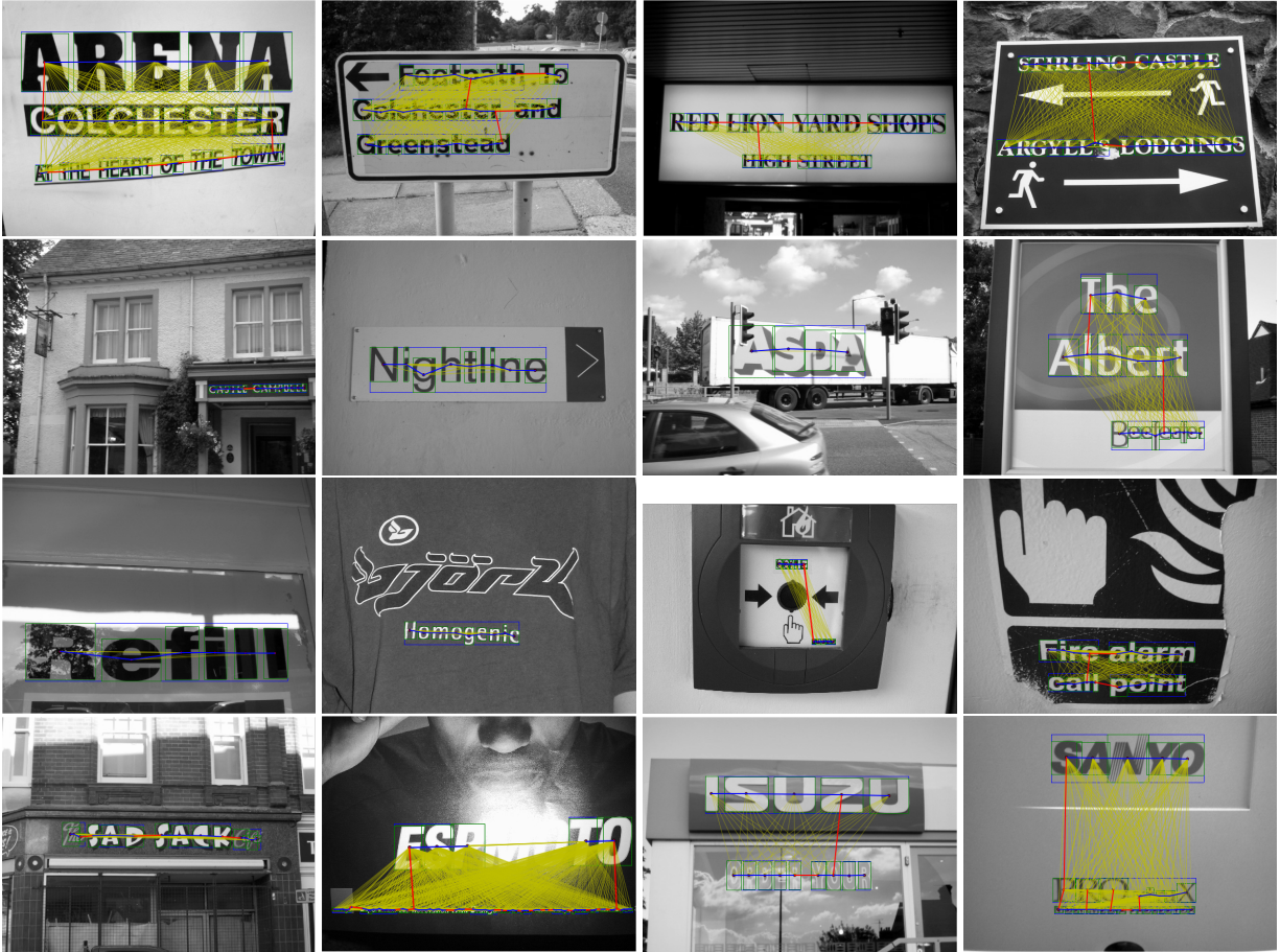
Figure 6.5: Segmentation using Word-Graph. The bounding box of characters are marked with green rectangles; the bounding box of words are marked with blue rectangles. Each character is a node in the graph model. Edges after MST trimming are used as training samples. The edges trimmed by MST are marked as yellow lines. Inter words edges are marked as red lines. The inner word edges are marked with blue lines.
