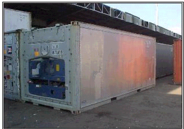
Figure 1. Reefer refrigeration system
