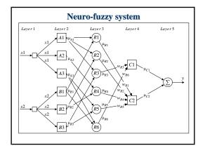
Each layer in the neuro-fuzzy system is associated with a particular step in the fuzzy inference process.
