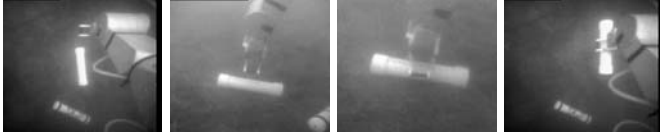
Fig. 2: Examples from a sequence of image fragments displayed to the operator during subsea trials [11]. Each image is 192x160 pixels, has been passed through contrast enhancement and JPEG compression/decompression. Note how the system automatically switches cameras while altering windowing and subsampling parameters.
